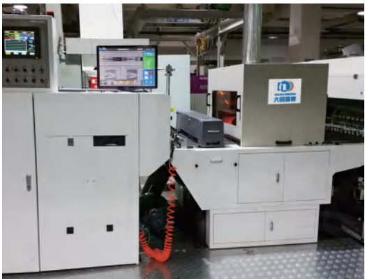
Webon - Inline inspection solutions for rotary die-cutting process
